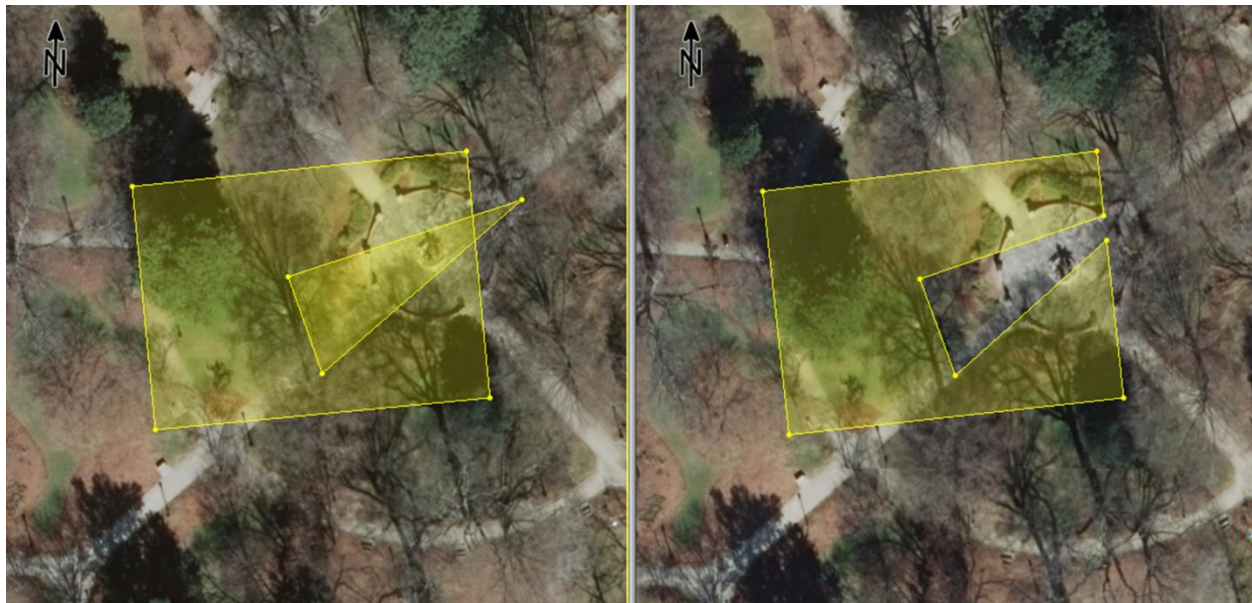
Figure 61. Using Boolean subtraction to carve complex shapes.
