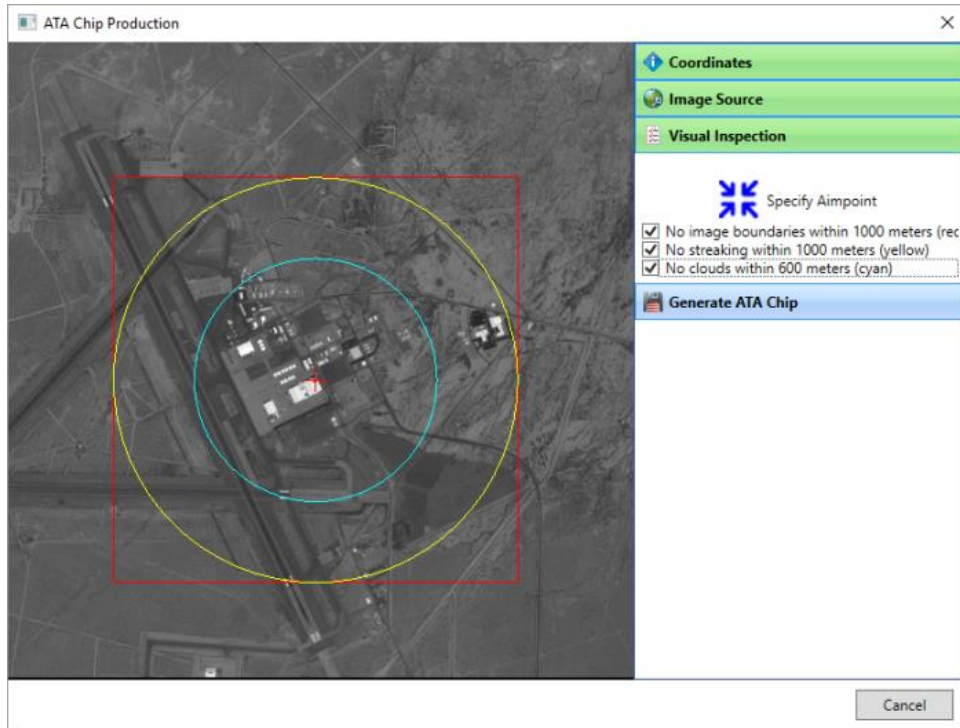
Figure 76. Stage 3: Specify the aimpoint and make visual checks for artifacts.
