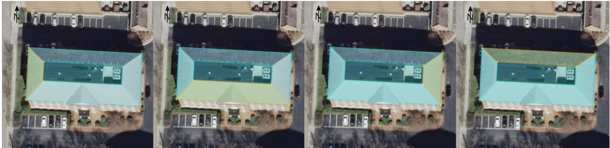
Figure 59. Using the snapping tool to build a roof structure by sections.
