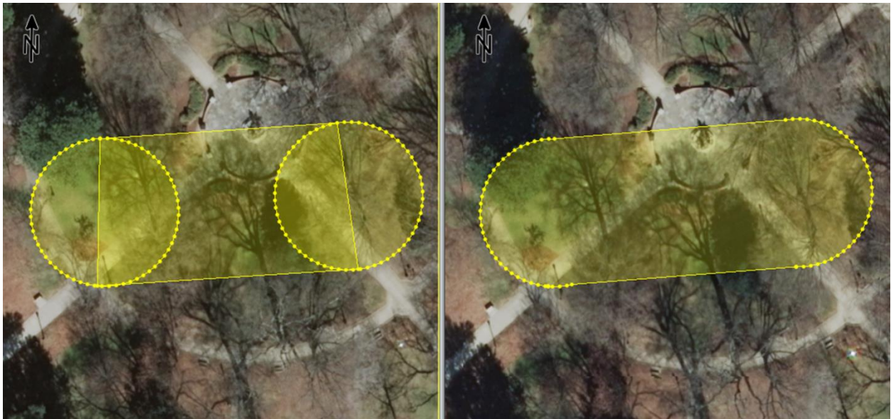
Figure 60. Combining multiple shapes using Boolean geometry.
